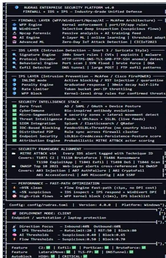
Fig. 2a: Rudras packet processing pipeline: each packet passes once through capture, fast-path validation, threat intelligence, IDS, DPI/WAF, AI behavioral scoring, and unified IPS enforcement, with structured logging at every stage.
