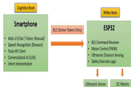
Fig. 1. Split-Brain System Architecture demonstrating the separation of cognitive and reflex layers.
