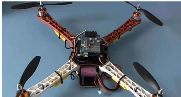
Fig 1, Image of drone system using Arduino
