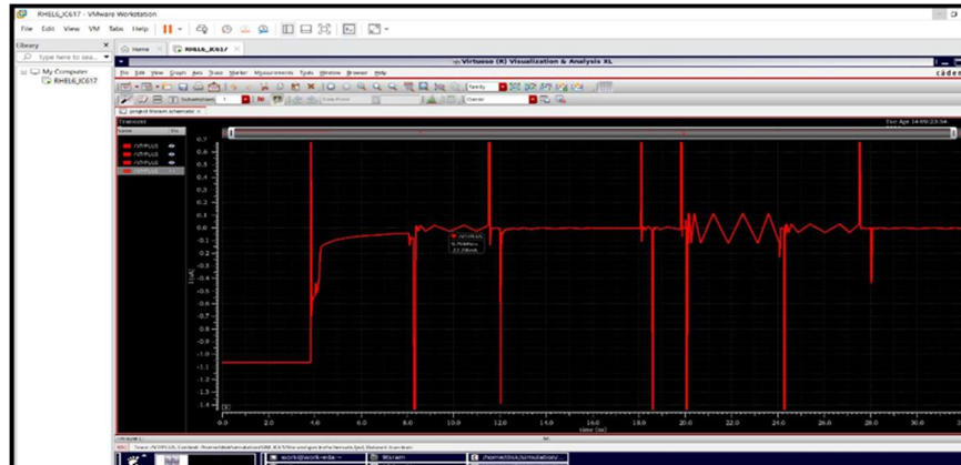
Figure 6.3 : leakage current waveform of the PR9T SRAM Cell
